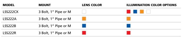
Replace "X" with **A** = Amber, **B** = Blue, **R** = Red, **W** = White Add "M" mounting extension to end of model for magnet mount
